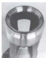
GTAW Weld Overlay Diesel Valve "Top"
